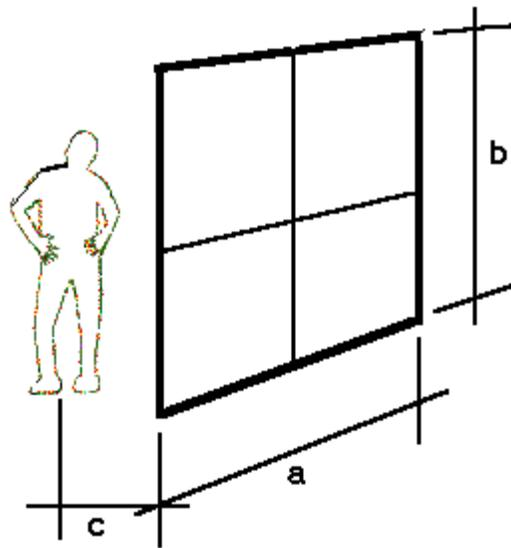
Figure 3. Occupant/window geometry used for view factor calculations.
